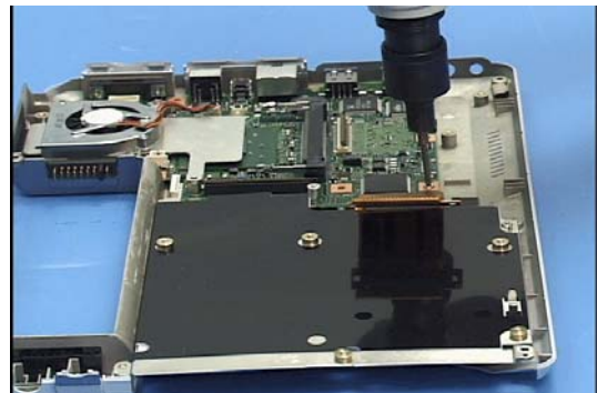
36. Remove 4 screws from the system board and lift it out.
