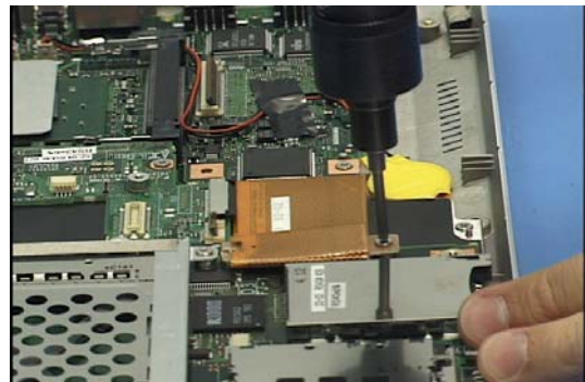
28. Remove 2 screws from the Expansion Card Daughterboard's cable and disconnect it.
