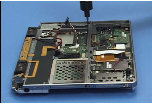
21. Remove 13 screws from the upper cover.
