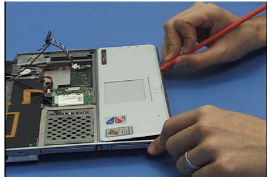
14. Use the plastic screwdriver to pry off the palm rest
