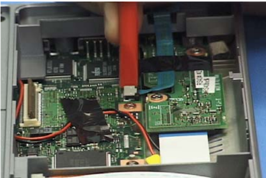
19. Disconnect the key lock LED cable, remove the tape from it and remove the LED board.
