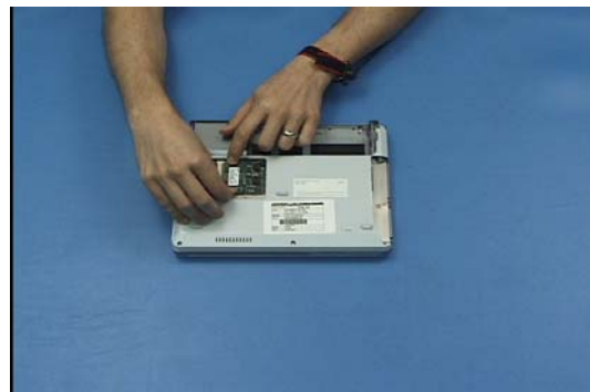
4. Remove the RAM by pressing out on the locking clips.
