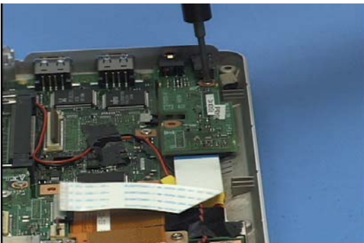
27. Remove 2 screws from the audio board, un-tape the microphone cable and remove them both.
