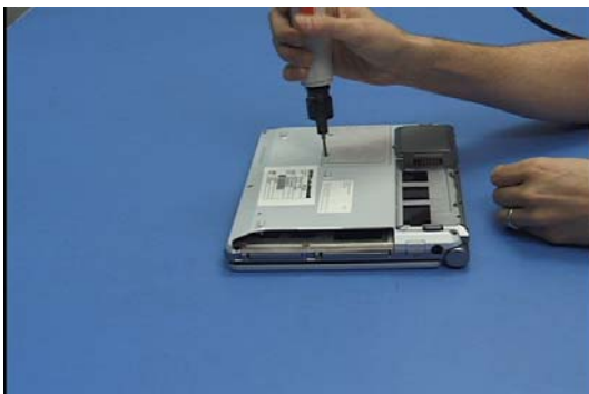
3. Extract 2 screws from the RAM cover and remove it.
