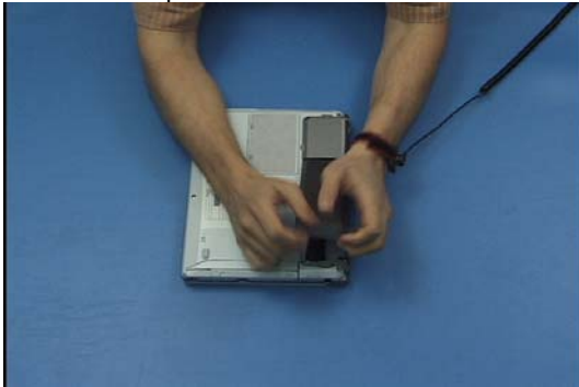
1. Turn the unit over and remove the battery.
