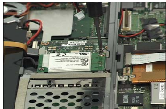
20. Remove 3 screws from the modem, disconnect the RJ11 cable from it and remove it.
